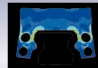
Example of roller slide deformation analysis
