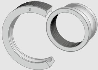
The adjacent bearings in the set are selected in the factory so that the maximum difference in bore or OD tolerance is within one third of the overall size tolerance. This is to ensure that once the bearings are fitted to the shaft and in the housing that the fits from bearing to bearing are fairly similar and thereby the load distribution within the bearing set is shared equally.
