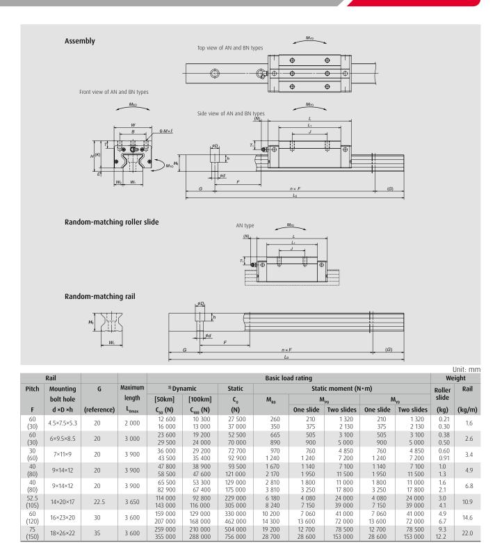
The random-matching type is available for the models of RA25 to RA65. The basic load rating comply with the ISO standard. (ISO 14728-1, 14728-2)  $C_{so}$ ; the basic dynamic load rating for 50 km rated fatigue life  $C_{100}$ ; the basic dynamic load rating for 100 km rated fatigue life
