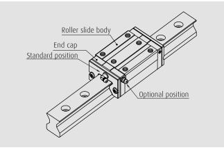
Fig. 8 Top and side lubrication hole positions
