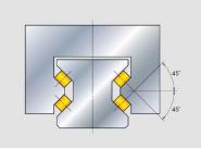
Balanced four-directional iso-load specifications
