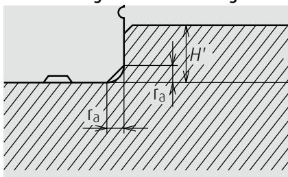
**Fig. 9 Shoulder for the rail datum surface**
