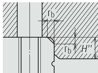
**Fig. 10 Soulder for the ball slide datum surface**
