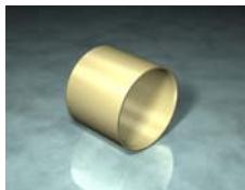
MP-210 is a thermoplastic material with fibres mixed with solid lubricants. This product has a low moisture absorption, good chemical resistance, low coefficient of friction, low wear against different shaft material; the best performance are with soft shaft material. Plain and flanged bearings are available as standard. Special shapes and sizes can be manufactured according to customer's requirements.
