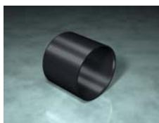
MP-300 is a thermoplastic material with fibres mixed with solid lubricants dedicated in those applications where traditional self-lubricating cannot guarantee the necessary resistance to the wear. This product has a good mechanical property and excellent self-lubricating property. Plain and flanged bearings are available as standard. Special shapes and sizes can be manufactured.
