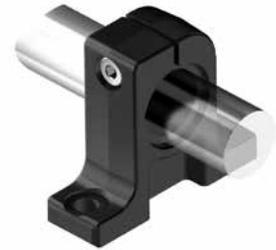
Type ASBM shaft blocks, manufactured from high-strength, extruded aluminum, provide either end or intermittent support in applications where loads are designed with a reference edge on one side of the base. This provides a surface parallel to the center of the shaft within  $\pm 0.025$  mm that can be used to simplify shaft alignment.
