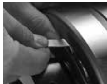
Fig. 97. Measure of RIC before installation.
