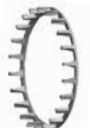
Fig. 46. Split, machined-brass, land-riding, finger-type cage.
