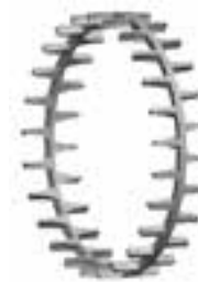
Fig. 45. One-piece, machined-brass, land-riding, finger-type cage.
