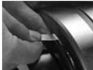
Fig. 91. Measure RIC before installation.
