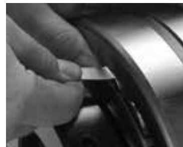
Fig. 95. Measure RIC before installation.
